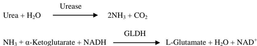
The rate of change of the absorbance difference between 340 nm and 405 nm is caused by the conversion of NADH to NAD<sup>+</sup> and is directly proportional to the amount of urea present in the sample.
