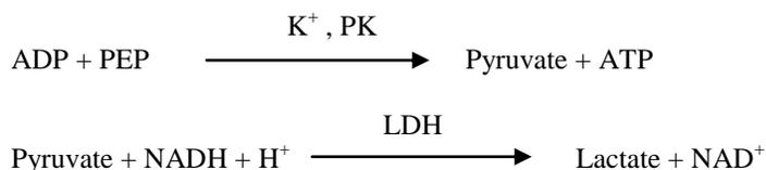
The rate of change in absorbance difference between 340 nm and 405 nm is due to the conversion of NADH to NAD<sup>+</sup> and is directly proportional to the amount of potassium in the sample.
