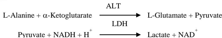
The rate of change of the absorbance difference between 340 nm and 405 nm is due to the conversion of NADH to  $\text{NAD}^+$  and is directly proportional to the amount of ALT present in the sample.
