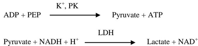
The rate of change in absorbance difference between 340 nm and 405 nm is due to the conversion of NADH to NAD<sup>+</sup> and is directly proportional to the amount of potassium in the sample.
