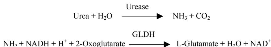
The rate of change of the absorbance difference between 340 nm and 405 nm is caused by the conversion of NADH to NAD<sup>+</sup> and is directly proportional to the amount of urea present in the sample.
